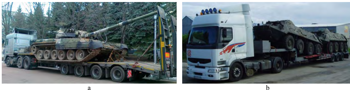
Fig. 1. Transportation on specialized platforms of heavy tracked (a) and wheeled (b) military vehicles
