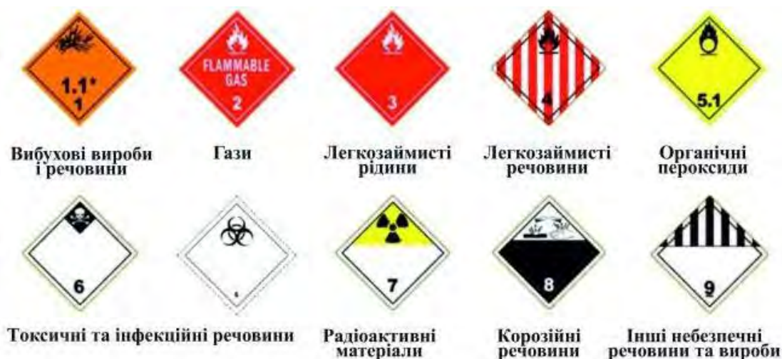
Figure 1 – Marking of dangerous goods
