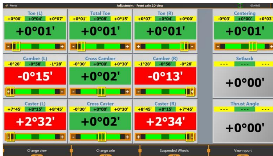
Figure 3 – Indications of wheel alignment angles
