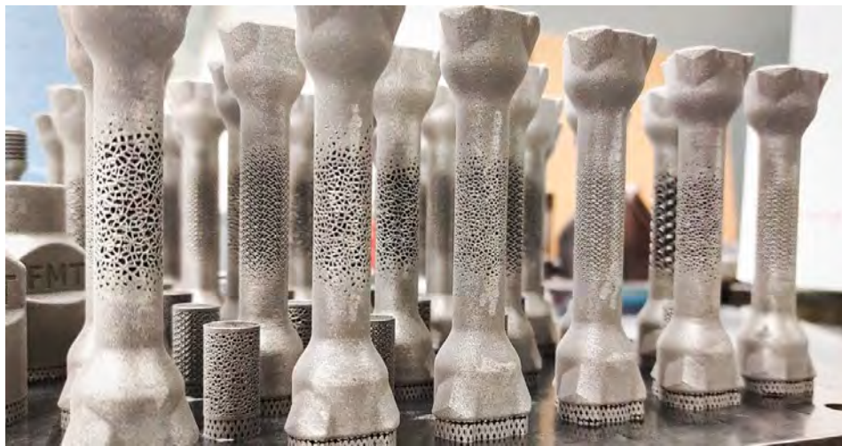
Picture 1 - A new type of orthopedic lightweight implants using metal 3D printing.
